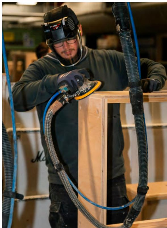
The Wood Mill is where the product cabinets begin to take shape, from cutting individual sheets of plywood to produce the tops, bottoms and sides of the cabinets to the hands-on gluing of cabinet joints and batten work, and finishing with the hand sanding, ensuring each piece resonates with the Marshall sound.
